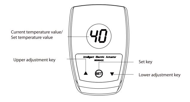
Set temperature:Press and hold the 'set key' for 3-5 seconds, the temperature of the LCD starts to jump at the current set temperature. Then press the 'upper adjustment key' or 'lower adjustment key' to adjust the set temperature value. After adjusting it, confirm the set temperature value after 15 seconds without operation.
